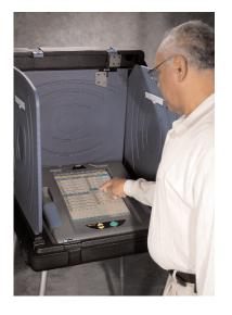
election is ever contested, **iVotronic**'s unique, patented recount system allows replication of the entire election process, including production of all ballot images for re-verification. Because each **iVotronic** unit is a self-contained election system, any malfunction in a single voter terminal has no effect upon the operation of other voter terminals in the precinct.
